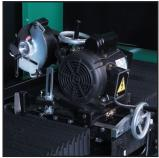
Single Point Infeed and a Patented Relief Indexing System allows for exact positioning of the grinding wheel and calibrated metal removal. The detachable "Auto-Index" relief finger assembly makes the transition from spin to relief easy and efficient.
