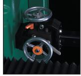
Positive, Vertical and Horizontal Reel Adjustments allows for easy alignment of the reel in the machine so the carriage travels perfectly parallel to reel.
