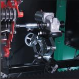
Independently Controlled, Reversible Variable Spin Drive provides optimum grinding performance, while the adjustable scissor jack allows for easy positioning of the quick disconnect spin drive coupler.
